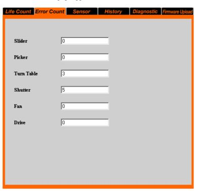
In the "Error Count" page, the number of times an operation was tried or an error occurred in the following specific parts are displayed.
